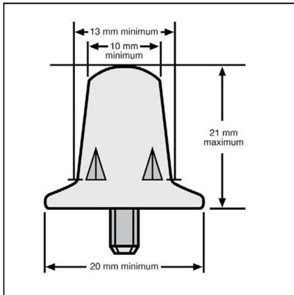
Also the minimum diameter values together with the maximum length value also defines a "comparator" stud/cleat, made in aluminium, that can be used in performance tests to evaluate alternatively shaped studs/cleats.
